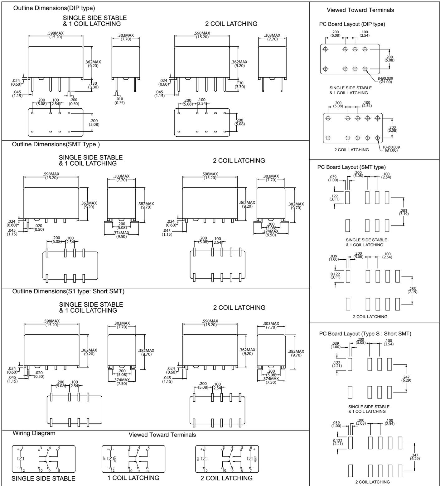
Dimensions in inch with millimeters in brackets below. Tolerance:  $\pm .010$ "
