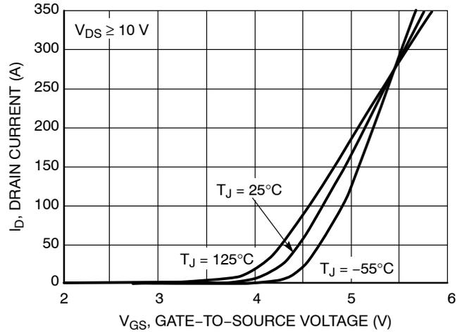
Figure 2. Transfer Characteristics
