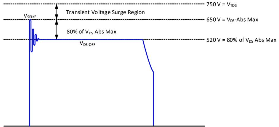
Fig. 28. QR flyback drain-to-source voltage stress diagram
