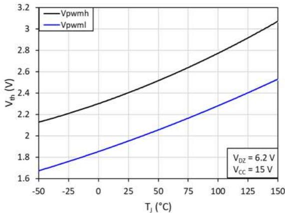
Fig. 7.  $V_{PWMH}$  and  $V_{PWMML}$  vs. junction temperature ( $T_J$ )
