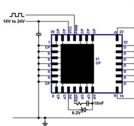
Fig. 18. Start-up circuit
