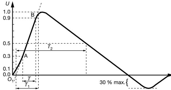
Front time:  $T_1 = 1.67 \times T = 1.2 \mu s \pm 30 \%$
