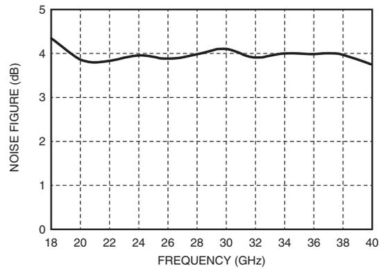
Note: Measured Performance Characteristics (Typical Performance at 25°C) Vd1 = 5V, Id1 = 45 mA
