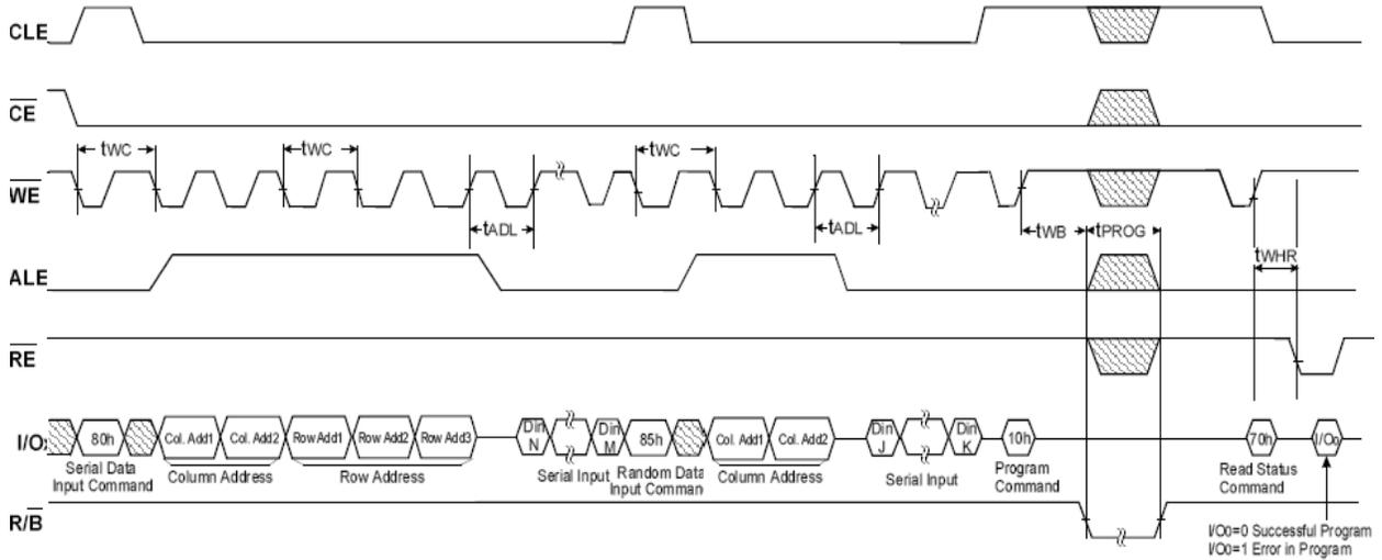
**Note:**  $t_{ADL}$  is the time from the WE# rising edge of final address cycle to the WE# rising edge of the first data cycle.
