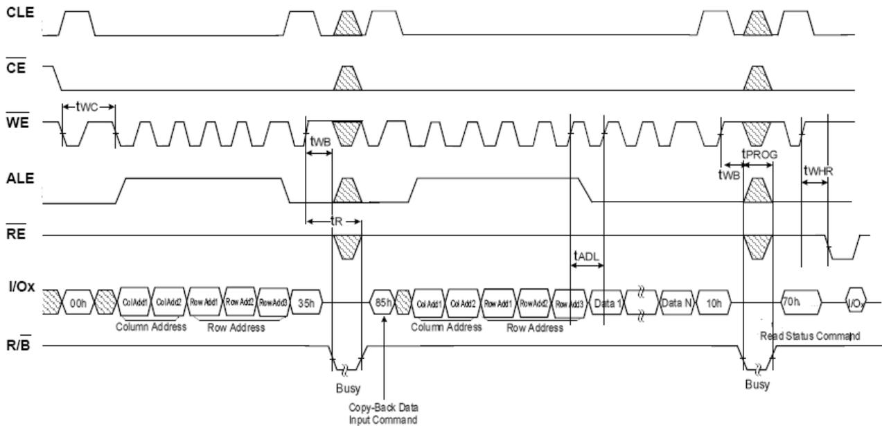
**Figure 6.12 Copy-Back Operation with Random Data Input**
