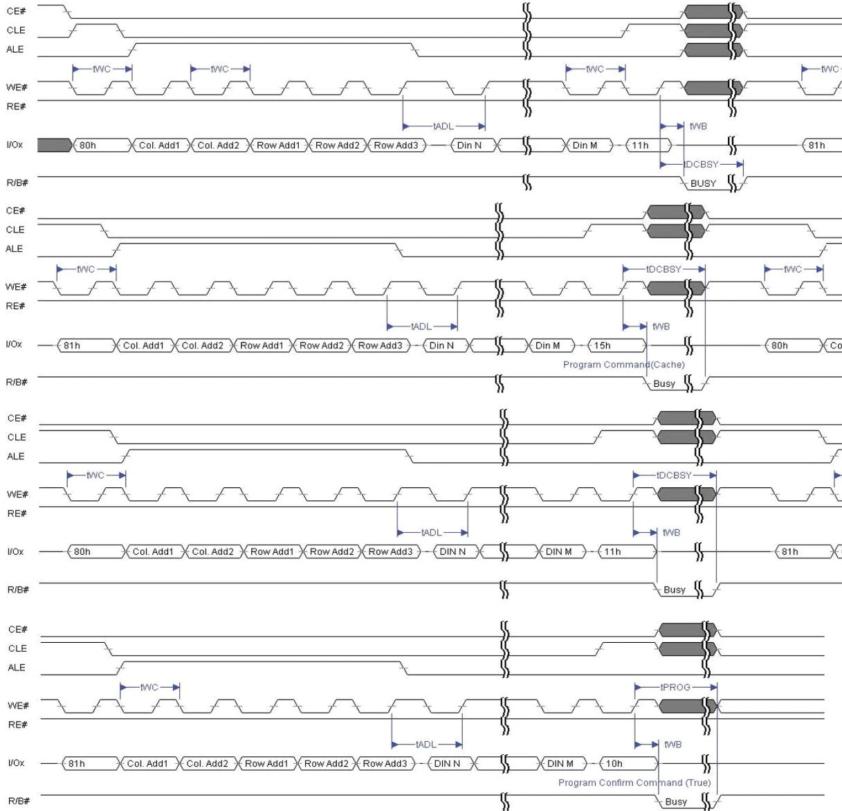
**Figure 6.20 Two-Plane Cache Program Operation**
