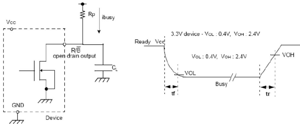
**R<sub>P</sub> vs t<sub>RHOH</sub> vs C<sub>L</sub>**
