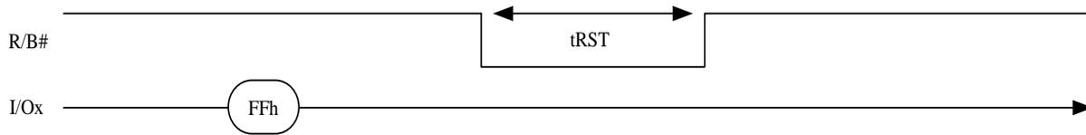
**Figure 8.10 Reset Operation**
