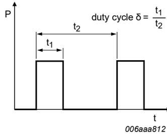
Fig. 17. Duty cycle definition
