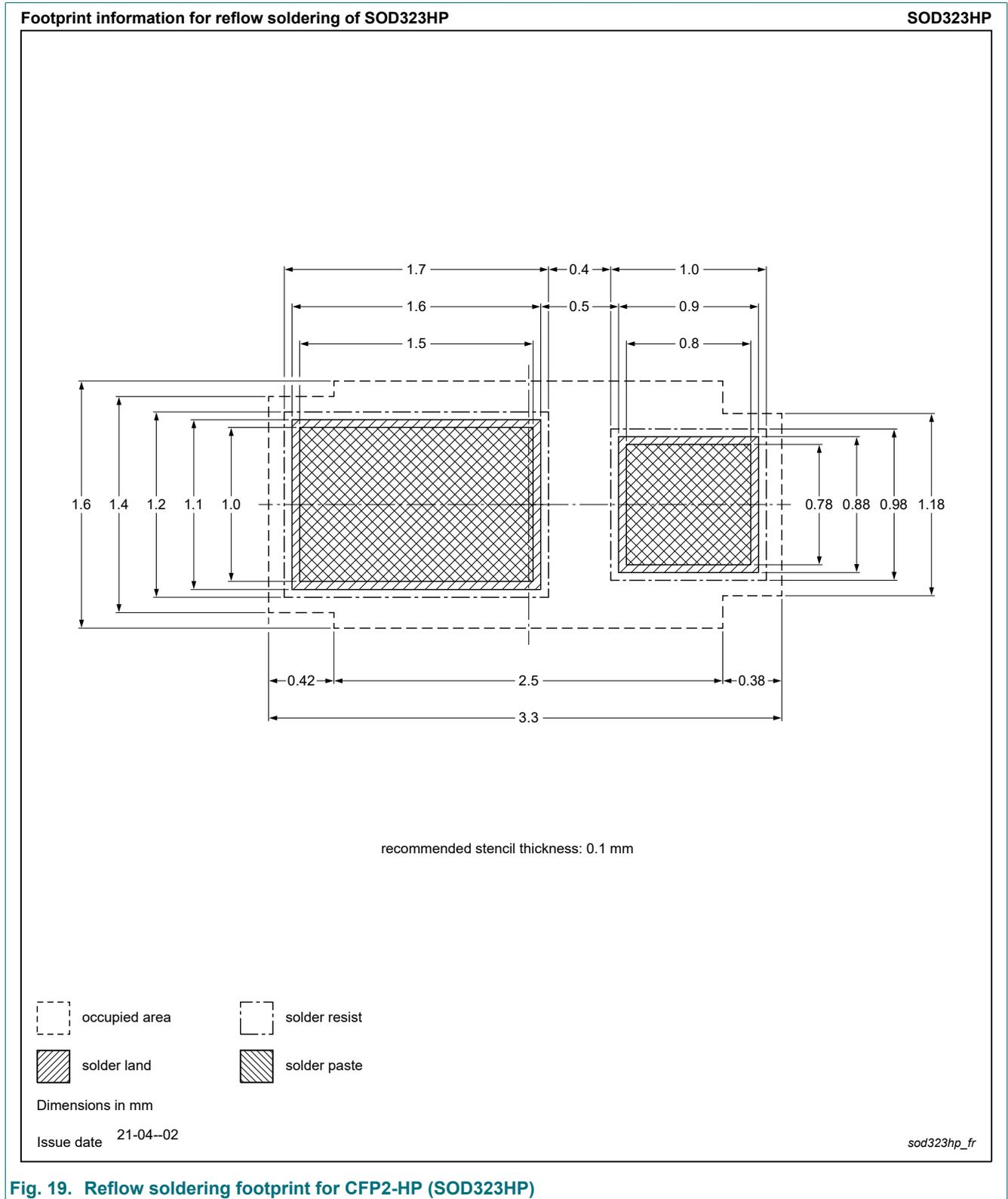
Fig. 19. Reflow soldering footprint for CFP2-HP (SOD323HP)
