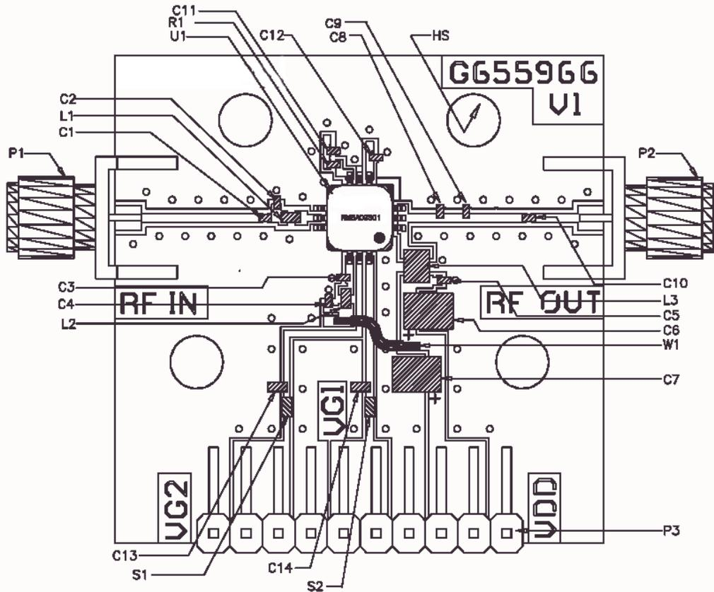
Figure 4. Layout of Test Evaluation Board (RMBA09501-TD, G657471)
