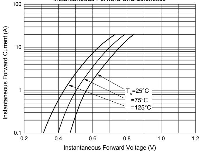
Fig. 4 - MBRB30150CTH Typical Instantaneous Forward Characteristics
