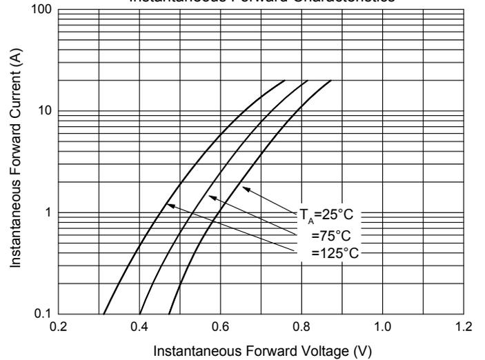
Fig. 5 - MBRB30200CTH Typical Instantaneous Forward Characteristics
