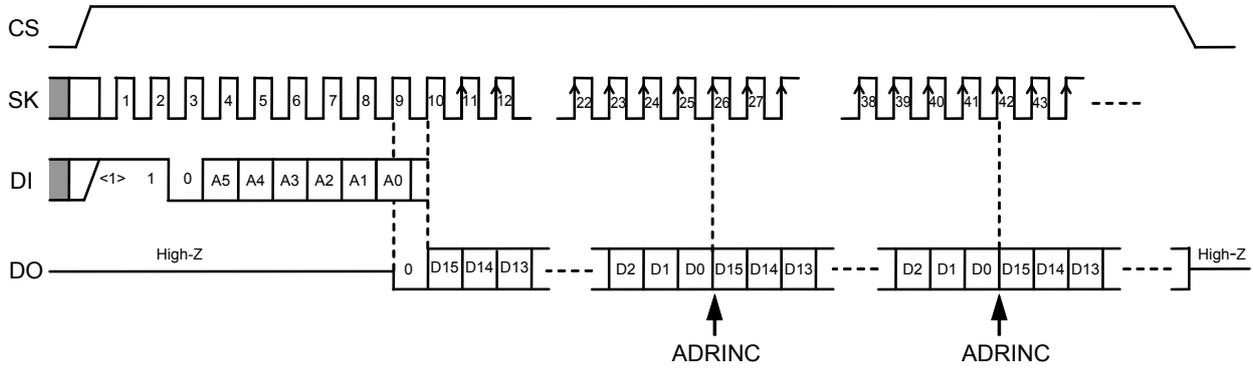
**Figure 2 Read Timing (S-93C46C)**
