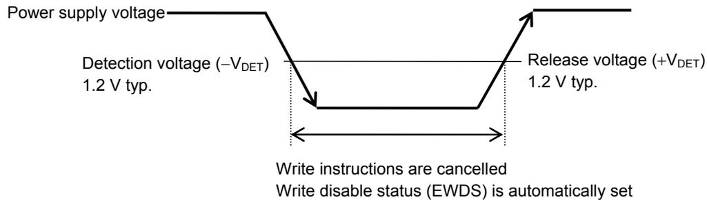
**Figure 20** Operation during the Low Power Supply Voltage
