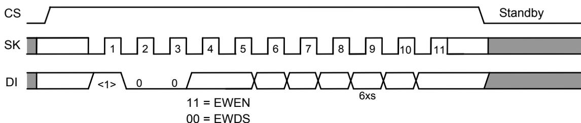
**Figure 18 Write Enable / Disable Timing (S-93C56C/66C)**
