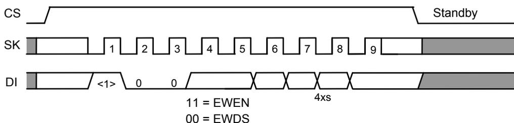
**Figure 17 Write Enable / Disable Timing (S-93C46C)**
