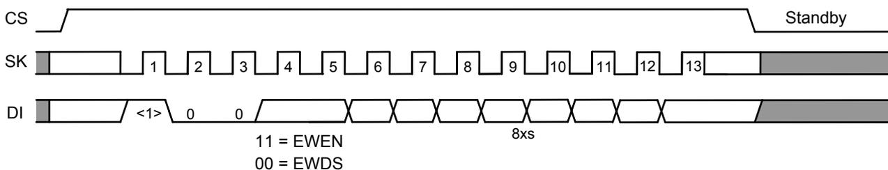
**Figure 19 Write Enable / Disable Timing (S-93C76C/86C)**
