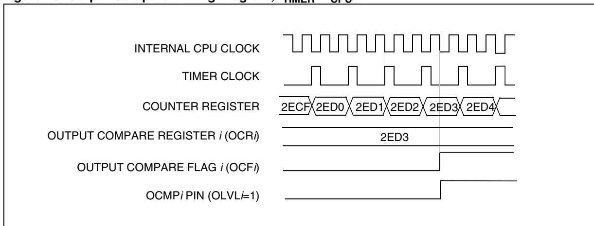
Figure 50. Output Compare Timing Diagram,  $f_{\text{TIMER}} = f_{\text{CPU}}/4$
