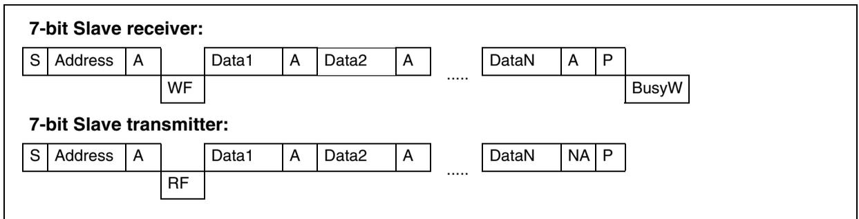
**Legend:** S=Start, P=Stop, A=Acknowledge, NA=Non-acknowledge, WF = WF event, WfX bit is set (with interrupt if ITWEx=1, after Stop or Restart conditions), cleared by reading the I2C3SSR register while no communication is ongoing.
