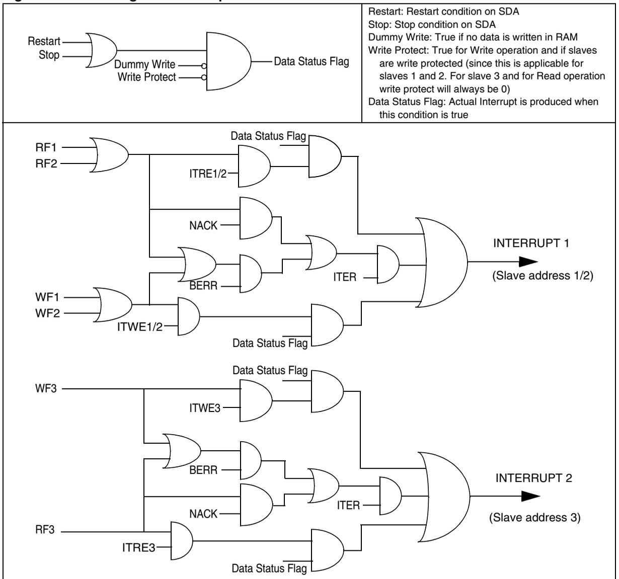
**Note:** Read/Write interrupts are generated only after stop or restart conditions. Figure 80 shows the conditions for the generation of the two interrupts.
