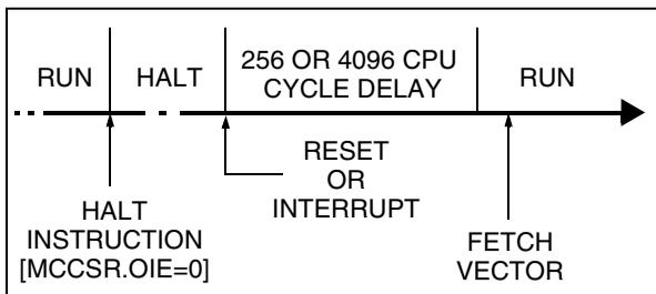
Figure 29. HALT Mode Flow-chart
