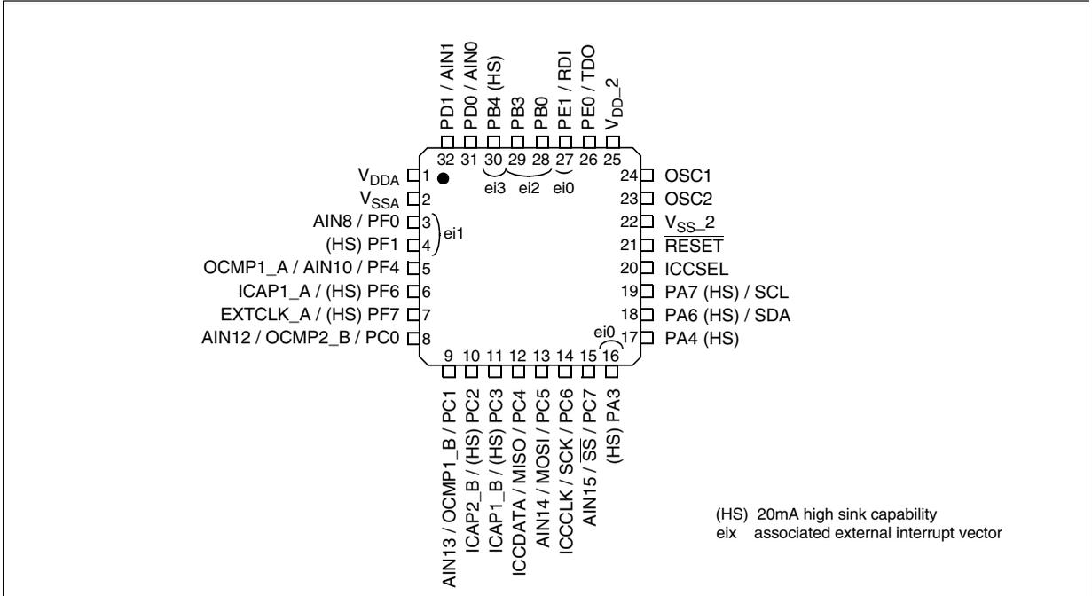
Figure 3. LQFP44 Package Pinout
