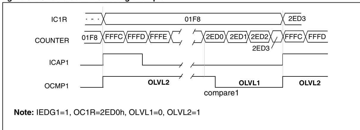
Figure 52. Pulse Width Modulation Mode Timing Example
