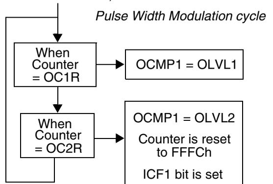
If OLVL1=1 and OLVL2=0 the length of the positive pulse is the difference between the OC2R and OC1R registers.
