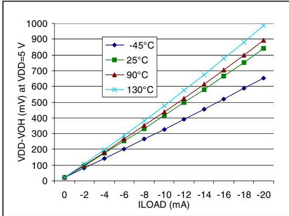
Figure 111. Typical  $V_{DD}-V_{OH}$  vs.  $V_{DD}$  (High Sink)
