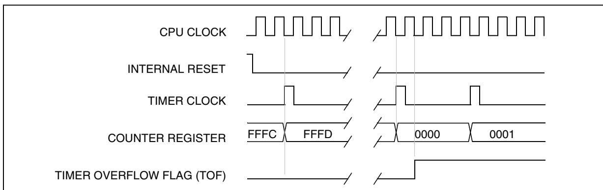
Figure 45. Counter Timing Diagram, internal clock divided by 8
