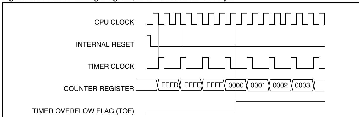
Figure 44. Counter Timing Diagram, internal clock divided by 4
