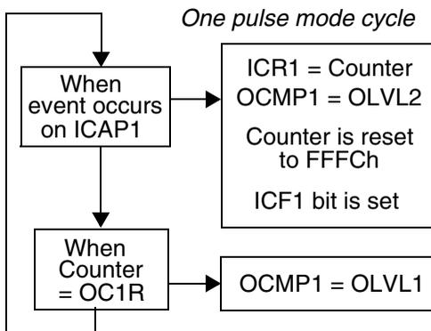
When a valid event occurs on the ICAP1 pin, the counter value is loaded in the ICR1 register. The counter is then initialized to FFFCh, the OLVL2 bit is output on the OCMP1 pin and the ICF1 bit is set.
