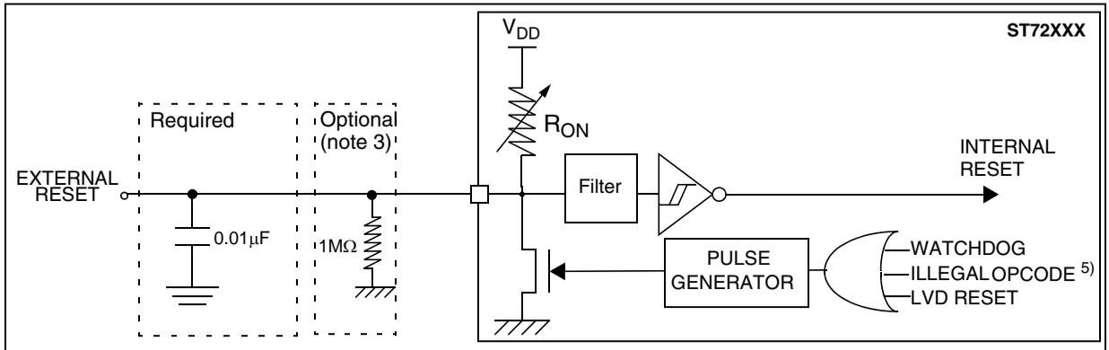
Figure 113.  $\overline{\text{RESET}}$  pin protection when LVD is disabled. <sup>1)</sup>
