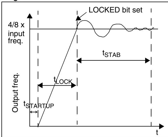
When the PLL is started, after reset or wakeup from Halt mode or AWUFH mode, it outputs the clock after a delay of  $t_{STARTUP}$ .
