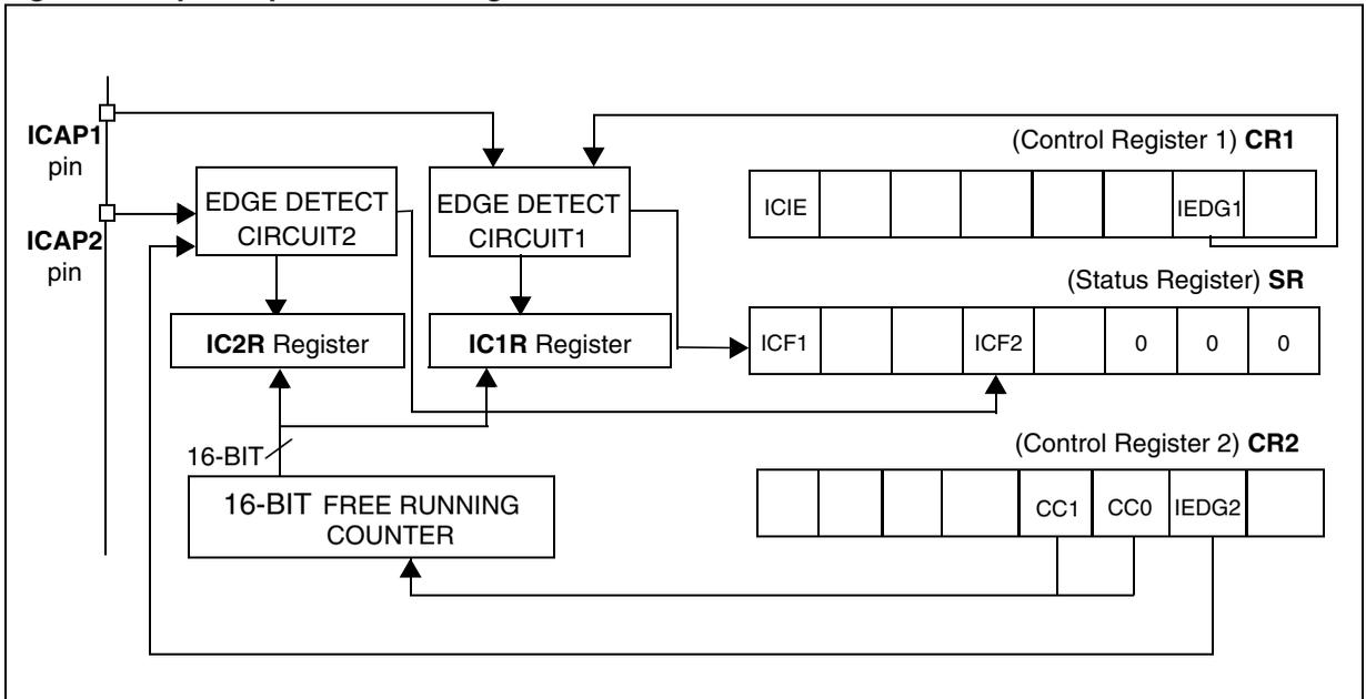
Figure 47. Input Capture Timing Diagram
