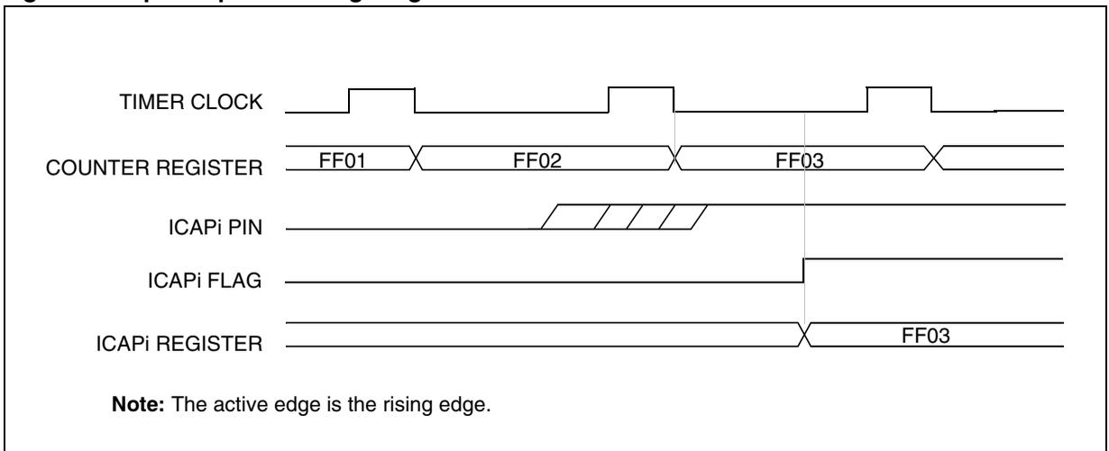
**Note:** The time between an event on the ICAPi pin and the appearance of the corresponding flag is from 2 to 3 CPU clock cycles. This depends on the moment when the ICAP event happens relative to the timer clock.
