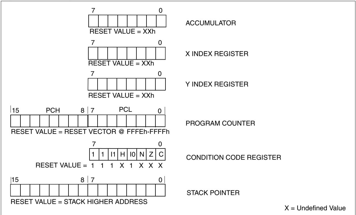
**CENTRAL PROCESSING UNIT (Cont'd)****Condition Code Register (CC)**
