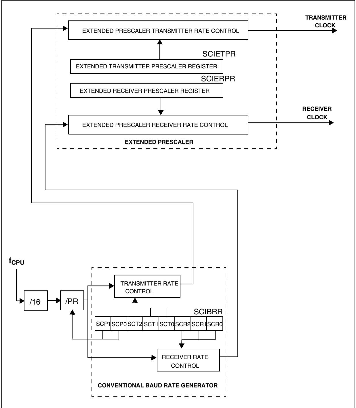
**SCI SERIAL COMMUNICATION INTERFACE** (Cont'd)**11.5.4.4 Conventional Baud Rate Generation**
