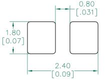
(For wave soldering, add 0.763 [0.030] to this dimension)
