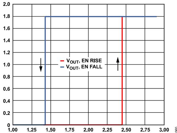
Figure 64. Typical  $V_{OUT}$  Response to EN Pin Operation
