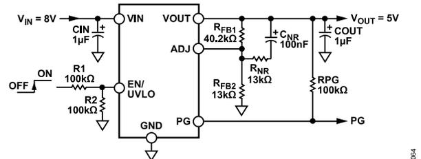
Figure 69. Noise Reduction Modification to Adjustable LDO
