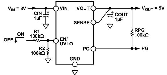
Figure 1. ADP7104 with Fixed Output Voltage, 5 V
