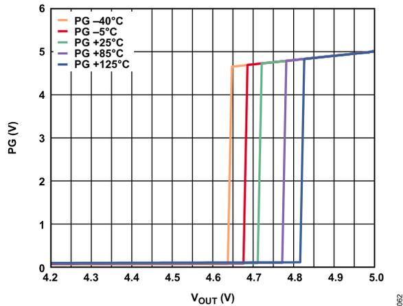
Figure 67. Typical Power-Good Threshold vs. Temperature,  $V_{OUT}$  Rising
