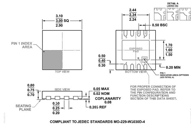
**Figure 80. 8-Lead Lead Frame Chip Scale Package [LFCSP]
