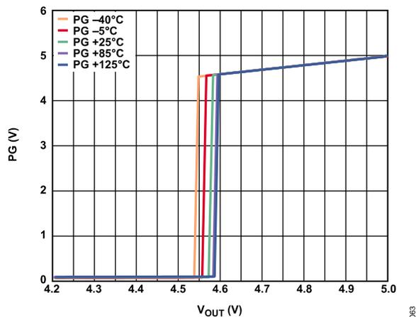
Figure 68. Typical Power-Good Threshold vs. Temperature,  $V_{OUT}$  Falling
