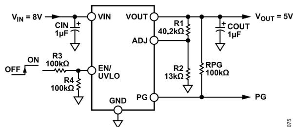
Figure 61. Typical Adjustable Output Voltage Application Schematic
