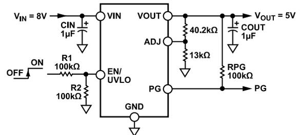
Figure 2. ADP7104 with Adjustable Output Voltage, 5 V
