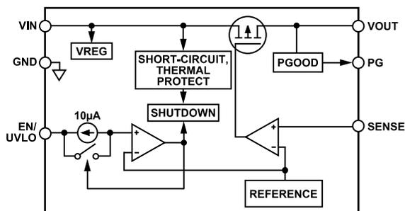
Figure 59. Fixed Output Voltage Internal Block Diagram
