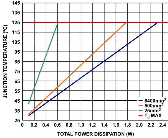
Figure 70. LFCSP, T<sub>A</sub> = 25°C
