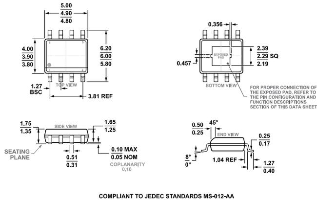
**Figure 81. 8-Lead Standard Small Outline Package, with Exposed Pad [SOIC\_N\_EP]
