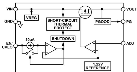
Figure 60. Adjustable Output Voltage Internal Block Diagram
