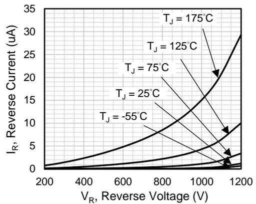
Fig.2 Reverse Characteristics
