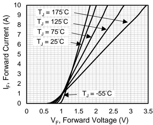
Fig.1 Forward Characteristics
