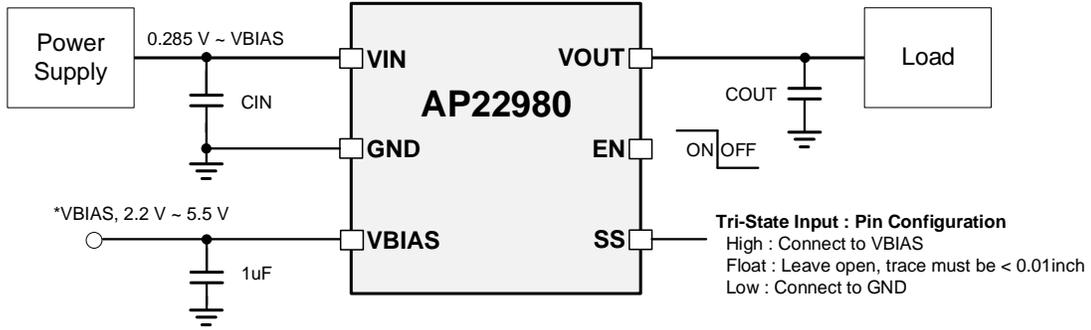
\* If VIN is higher than 2.2V then VBIAS pin can be connected to VIN.
