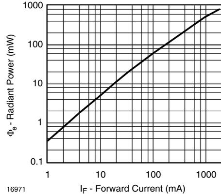
Fig. 6 - Radiant Power vs. Forward Current
