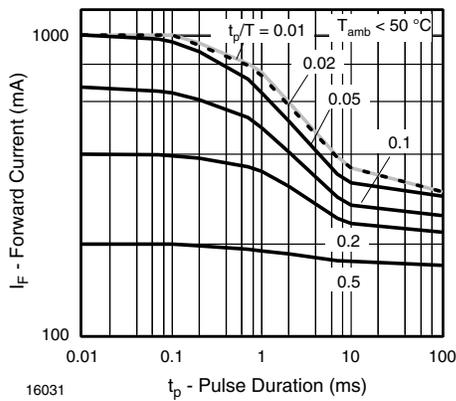
Fig. 4 - Pulse Forward Current vs. Pulse Duration
