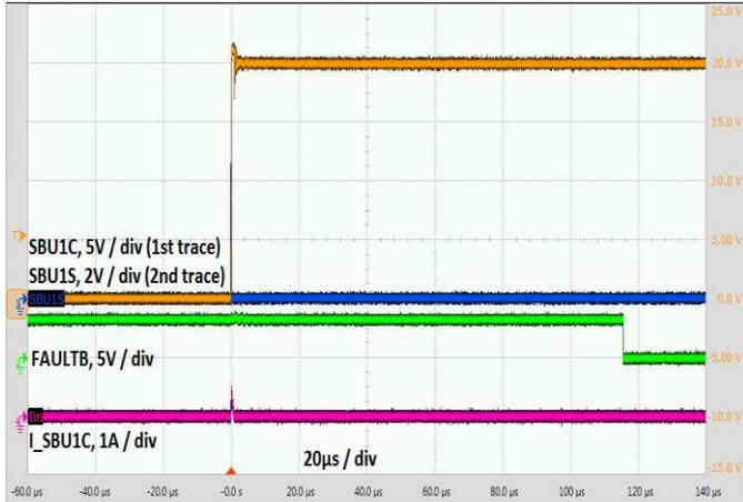
Figure 15. SBU1C Short to 20V V<sub>BUS</sub>
