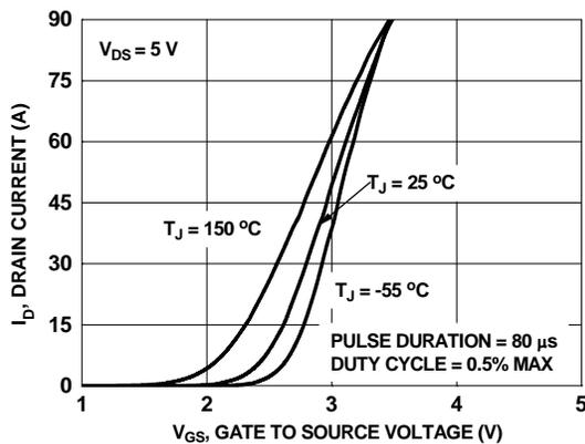
**Figure 5. Transfer Characteristics**
