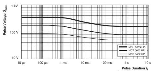
Maximum pulse voltage, single and continuous pulses; applicable if  $\hat{P} \leq \hat{P}_{\text{max}}$ ; for permissible resistance change  $\pm$  (0.5 % R + 0.05  $\Omega$ )
