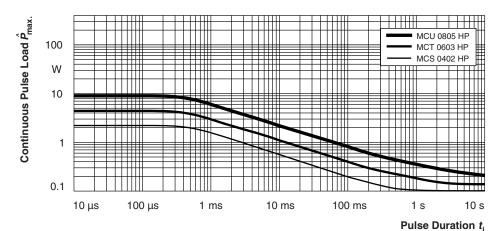
Maximum pulse load, continuous pulses; applicable if  $\overline{P} \leq P$  ( $\mathcal{G}_{amb}$ ) and  $\hat{U} \leq \hat{U}_{max}$ ; for permissible resistance change  $\pm$  (0.5 % R + 0.05  $\Omega$ )
