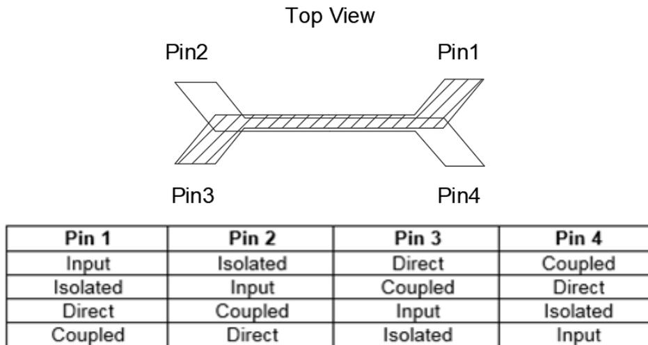
Note: The direct port has a DC connection to the input port and the coupled port has a DC connection to the isolated port.
