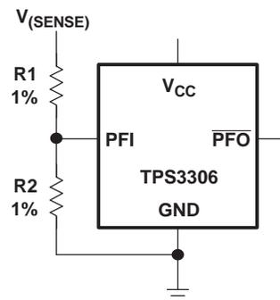
$$V_{PFI,trip} = 1.25\text{ V} \times \frac{R_1 + R_2}{R_2}$$
