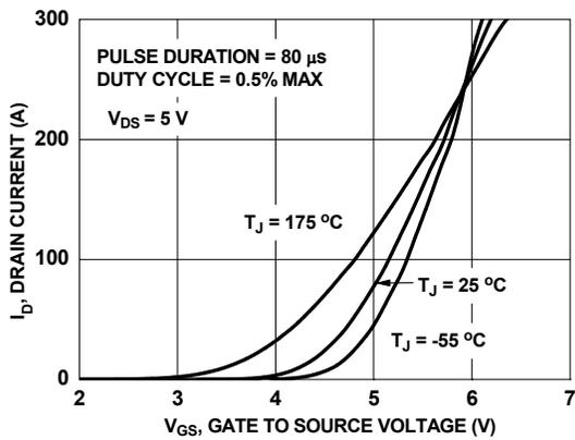
**Figure 5. Transfer Characteristics**
