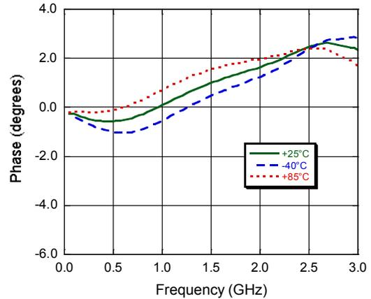
**Phase - 31 dB Attenuation vs. Frequency**
