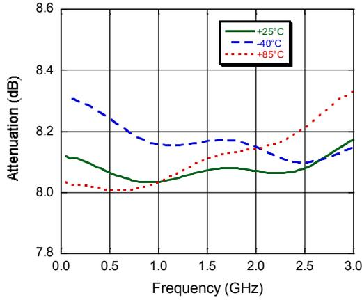
**Attenuation - 16 dB Bit vs. Frequency**
