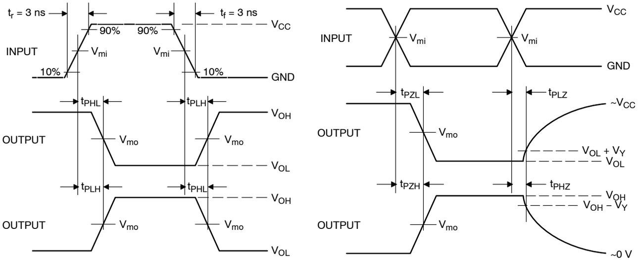
**Figure 4. Switching Waveforms**
