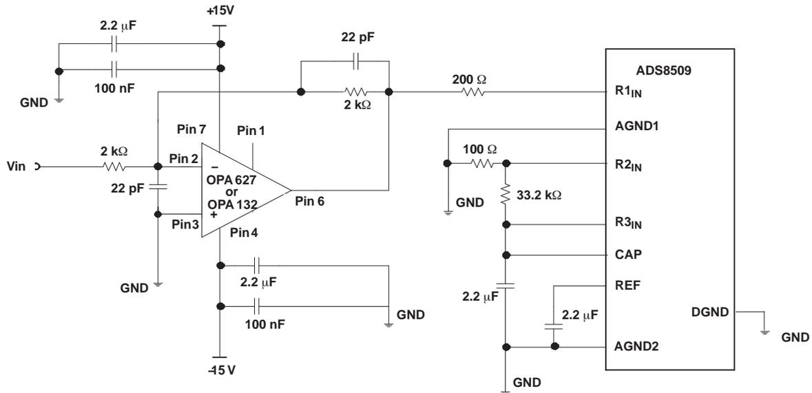
Figure 28. Typical Driving Circuitry ( $\pm 10$  V, No Trim)
