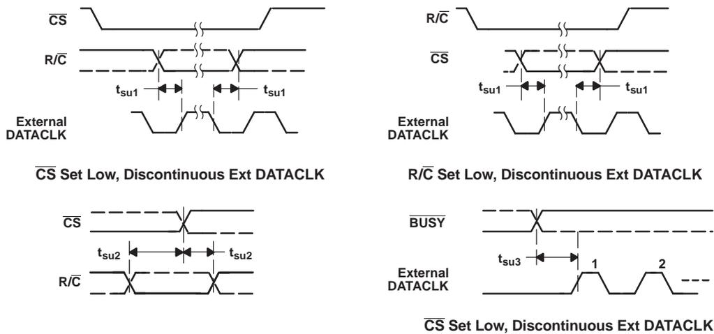
**Figure 1. Critical Timing**
