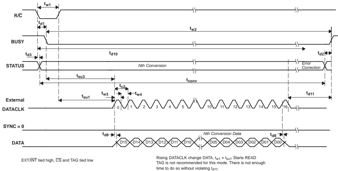
Figure 5. Read During Conversion (Discontinuous External DATACLK)
