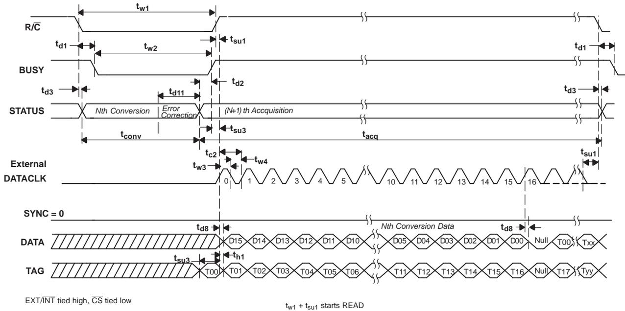
Figure 4. Read After Conversion (Discontinuous External DATACLK)
