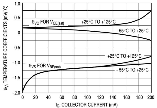
Figure 17. Temperature Coefficients
