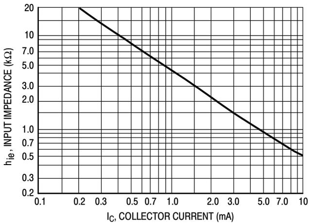
Figure 12. Input Impedance
