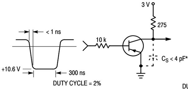
Figure 2. Delay and Rise Time Equivalent Test Circuit
