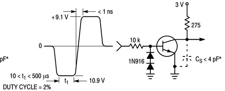
Figure 3. Storage and Fall Time Equivalent Test Circuit
