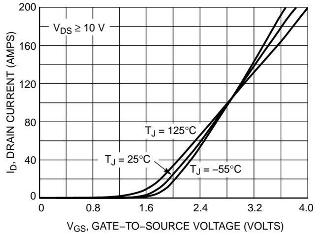
Figure 2. Transfer Characteristics
