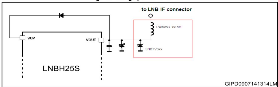
For this purpose, the use of the LNBTVSxx surge protection diodes specifically designed by ST is recommended. The selection of the LNBTVSxx diodes should be based on the maximum peak power dissipation supported by the diode (see the LNBTVS datasheet for further details).
