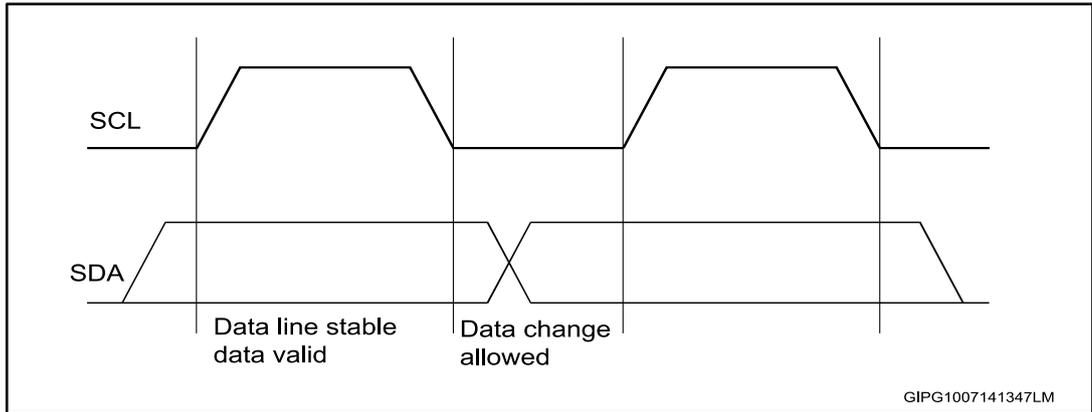
Figure 9: Timing diagram of I<sup>2</sup>C bus
