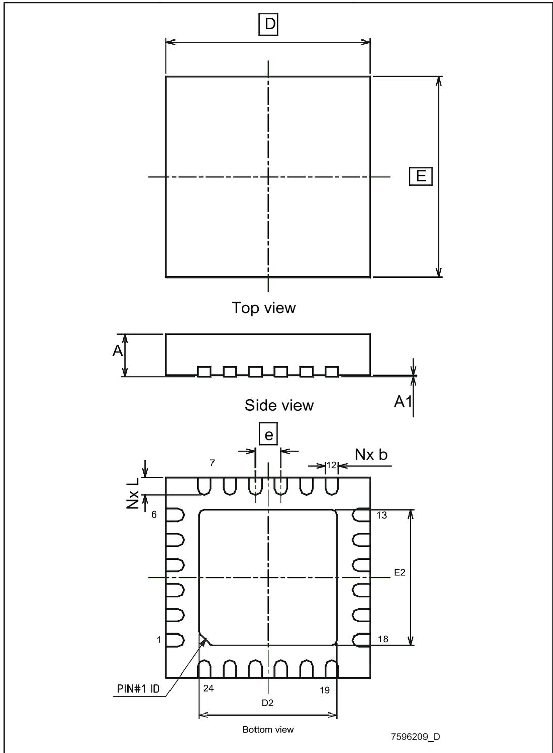
Table 20: QFN24L (4x4 mm) mechanical data
