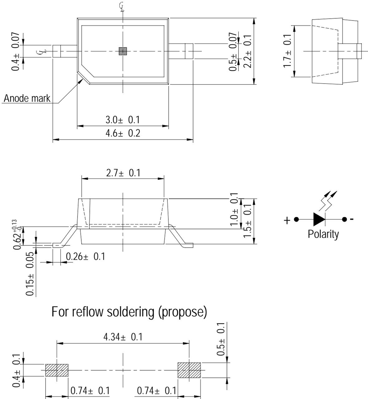
For reflow soldering (propose)
