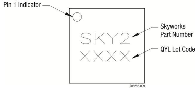
Figure 9. SKY59272-707LF Typical Part Markings (Top View)
