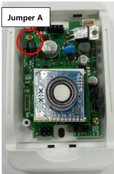
4 ~ 20mA is default (2 ~ 10VDC or 0 ~ 20mA or 0 ~ 10VDC is selectable with jumper setting change)
