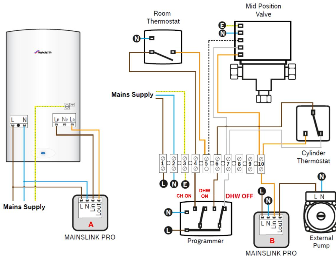
This system provides two functions, Switching of the Pump from the boiler and Switching of the Boiler from the wiring Centre.
