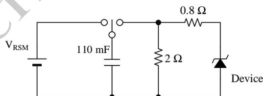
Figure 2. Surge Reverse Voltage Measurement Circuit (JASO A-1)
