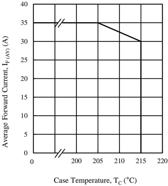
Figure 3. Power Dissipation Curves<sup>(2)</sup>
