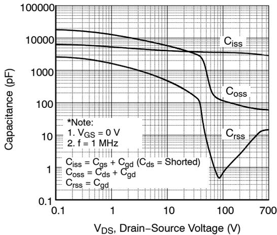
Figure 5. Capacitance Characteristics
