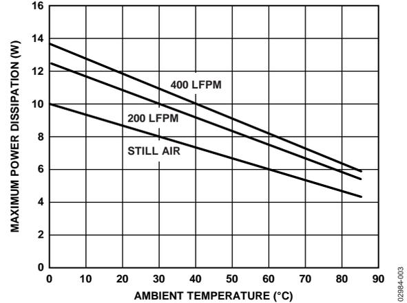
Figure 7. Maximum Power Dissipation vs. Ambient Temperature
