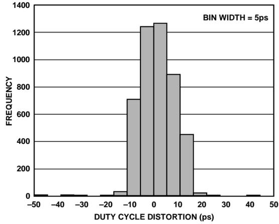
Figure 15. Duty Cycle Distortion Distribution
