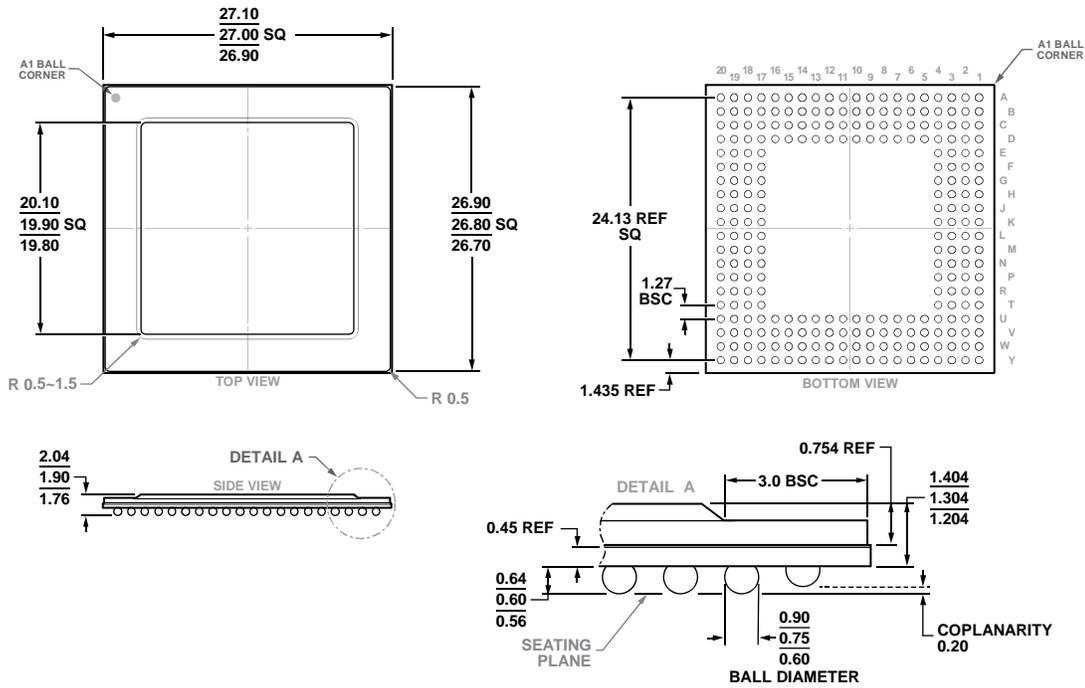
Figure 38. 256-Ball Ball Grid Array, Thermally Enhanced [BGA\_ED]
