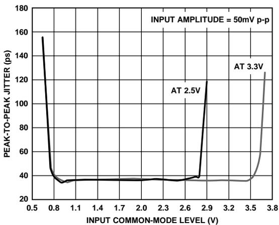
Figure 23. Peak-to-Peak Jitter vs. Input Common-Mode Level
