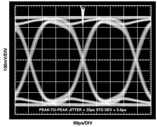
Figure 19. Crosstalk, 3.2 Gbps, Attack Signal Off (See Figure 33)
