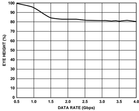
Figure 16. Eye Height vs. Data Rate
