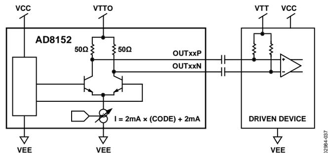
Figure 36. AC Coupling Output Signal from AD8152
