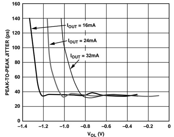
Figure 25. Peak-to-Peak Jitter vs.  $V_{OL}$  (Relative to VCC)
