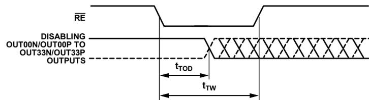
Figure 6. Asynchronous Reset
