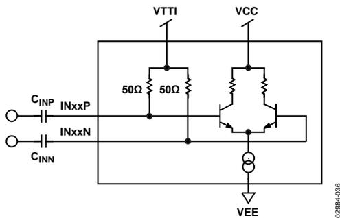
Figure 35. AC Coupling Input Signal from AD8152
