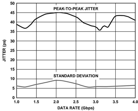
Figure 17. Jitter vs. Data Rate
