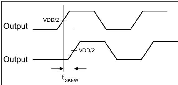
**FIGURE 1-2:** Output-to-Output Skew.
