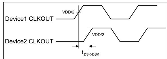
**FIGURE 1-5:** Device-to-Device Skew.
