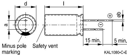
Safety vent for diameter  $\geq 8$  mm.
