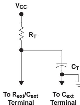
**Figure 2. Timing-Component Connections**
