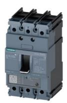
circuit breaker 3VA5 UL frame 125 3-pole, starter protection TM120M, AM, In=10A without overload protection short-circuit protection li=3...7 x In nut keeper kit on both sides
