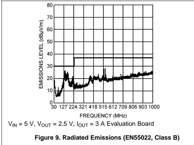
**Figure 9. Radiated Emissions (EN55022, Class B)**
