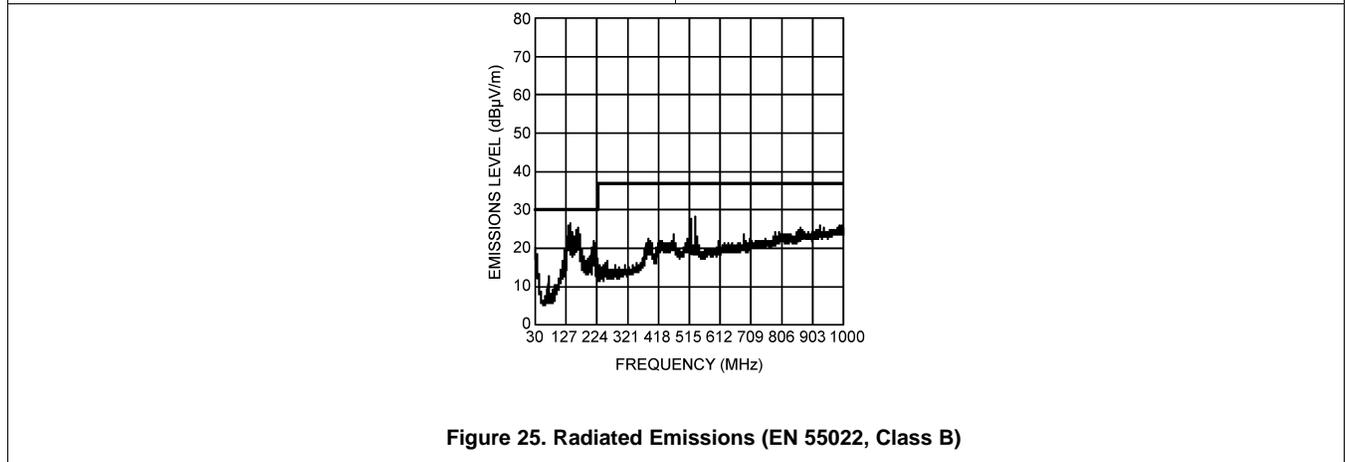
Figure 25. Radiated Emissions (EN 55022, Class B)
