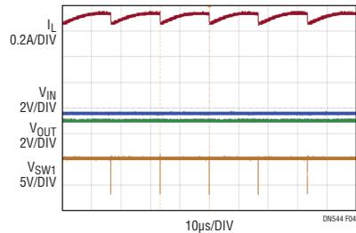
Figure 4. Dropout Performance at  $I_{OUT} = 1.5A$
