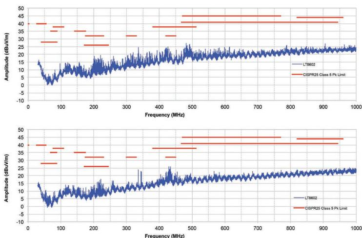
Figure 2. Radiated EMI Performance (CISPR25, Class 5, Peak Detector), 14VIN, 1A at All Outputs, Switching Frequency = 2MHz
