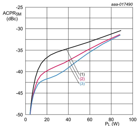
$V_{DS} = 28\text{ V}$ ;  $I_{Dq} = 650\text{ mA}$  (main);  $V_{GS(amp)peak} = 0.5\text{ V}$ .
