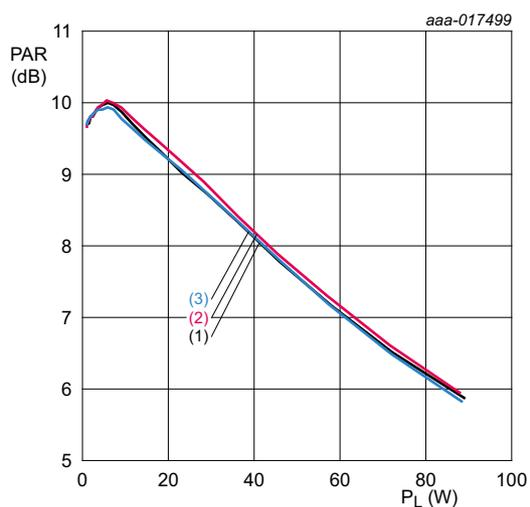
$V_{DS} = 28\text{ V}$ ;  $I_{Dq} = 650\text{ mA}$  (main);  $V_{GS(amp)peak} = 0.5\text{ V}$ .
