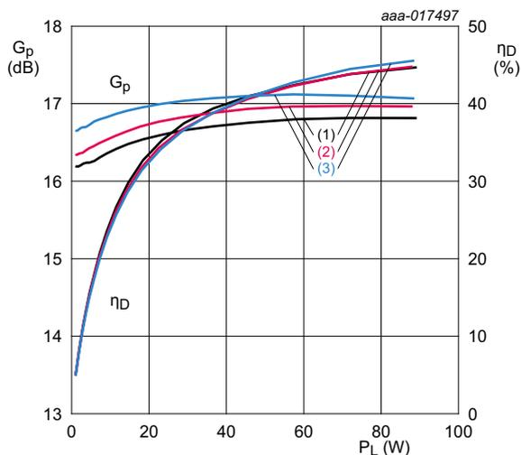
$V_{DS} = 28\text{ V}$ ;  $I_{Dq} = 650\text{ mA}$  (main);  $V_{GS(amp)peak} = 0.5\text{ V}$ .
