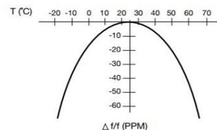
*To determine frequency stability, use parabolic curvature. For example: What is the stability at 45 $^{\circ}C$ ?*
