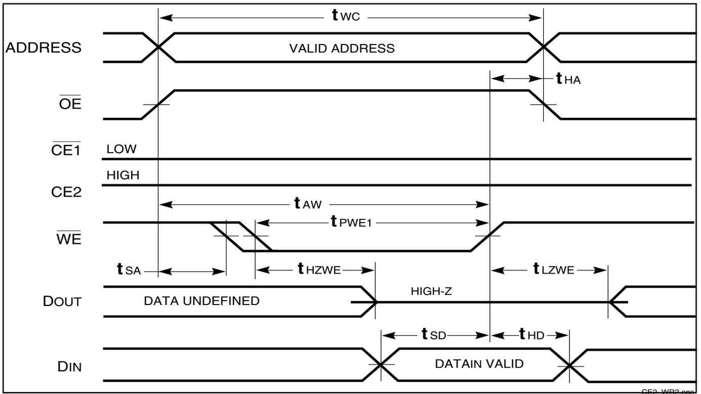
**WRITE CYCLE NO. 3<sup>(1)</sup>** ( $\overline{WE}$  Controlled:  $\overline{OE}$  IS LOW DURING WRITE CYCLE)
