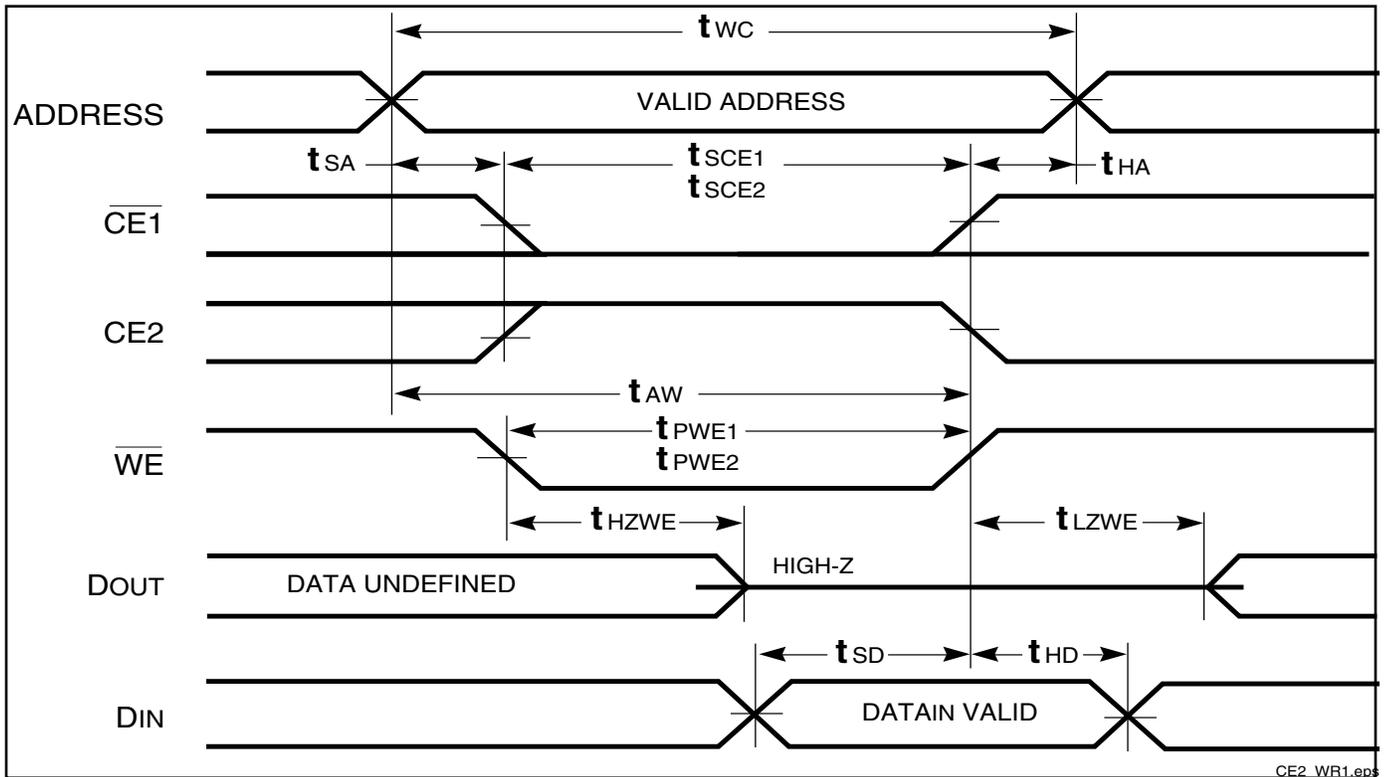
**WRITE CYCLE NO. 2<sup>(1)</sup>** ( $\overline{WE}$  Controlled:  $\overline{OE} = \text{HIGH during Write Cycle}$ )
