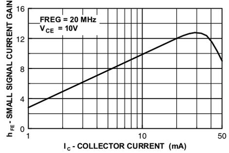
**Figure 10. Small Signal Current Gain vs. Collector Current**
