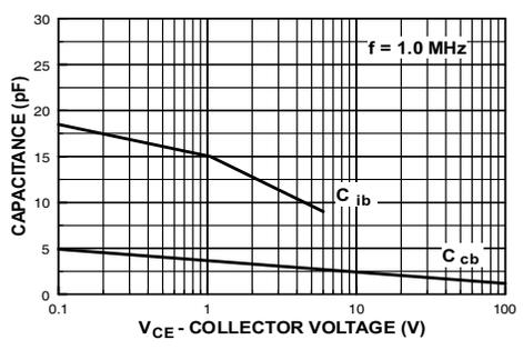
**Figure 9. Input and Output Capacitance vs. Reverse Voltage**
