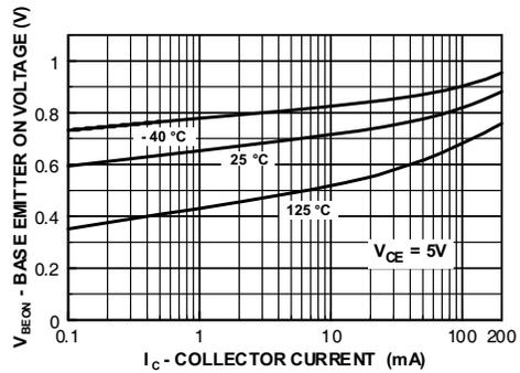
Figure 6. Base-Emitter On Voltage vs. Collector Current
