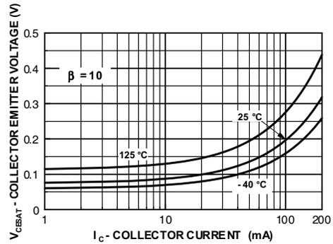
Figure 4. Collector-Emitter Saturation Voltage vs. Collector Current
