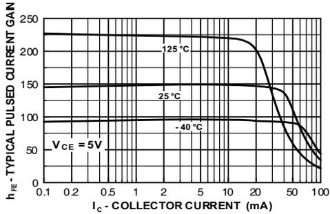
Figure 3. Typical Pulsed Current Gain vs. Collector Current
