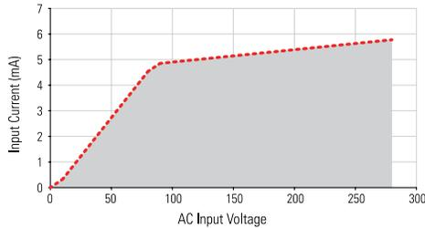
Input Current vs Input Voltage
