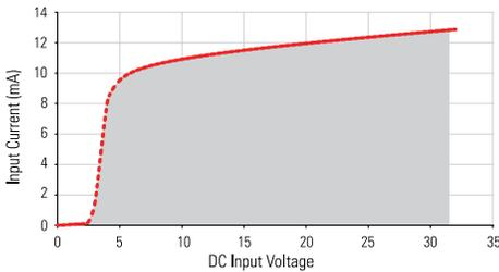
Input Current vs Input Voltage
