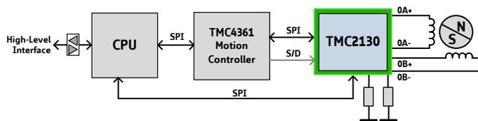
The CPU initializes the TMC4361 motion controller and the TMC2130. Thereafter, it sends target positions to the TMC4361. Now, the TMC4361 takes control over the TMC2130. Combining the TMC4361 and the TMC2130 offers diverse possibilities for demanding applications including servo drive features.
