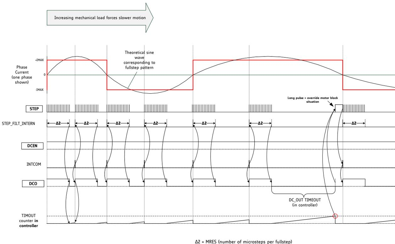
Figure 18.5 DCO Interface to motion controller – step generator stops when DCO is asserted
