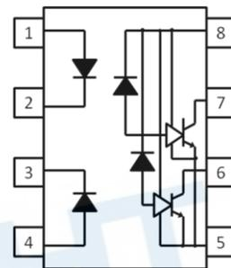
A 0.1μF bypass capacitor must be connected between pins 8 and 5 \*3
