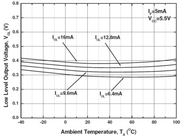
Figure 3. Low Level Output Current vs Ambient Temperature
