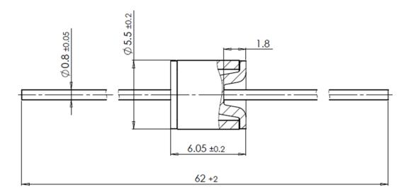
Drawing of new MF welding design:
