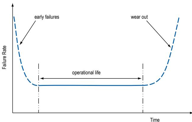
The failure rate is derived from our periodic test results. The failure rate ( $\lambda R$ ) is, therefore, only given at test temperature for life tests. An estimation is also given at 40°C. The expected failure rate for this capacitor range is based on our periodic test results for capacitors with structural similarity. Failure rate is frequently quoted in FIT (Failures In Time) where 1 FIT = 1x 10<sup>-9</sup> failures per hour. Failure rates include both catastrophic and parametric failures.
